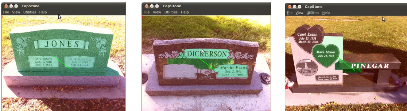
Figure 4. Graph cuts based on simple seeding lines
