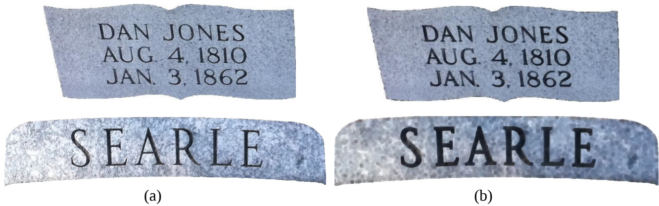
Figure 5. (a) Images of headstone information inscribed on noisy stone. (b) Same images after passing through a median filter
