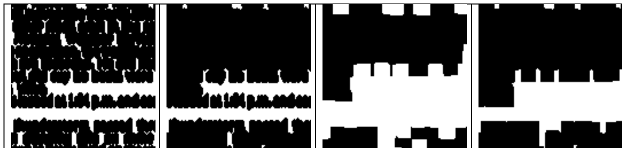
Figure 7: From left to right: Results from 2-point erosion performed on the word blobs; Results after from inverse image holes filling; Results from image dilation; Results from image erosions and final image used from creating primary article zones.
