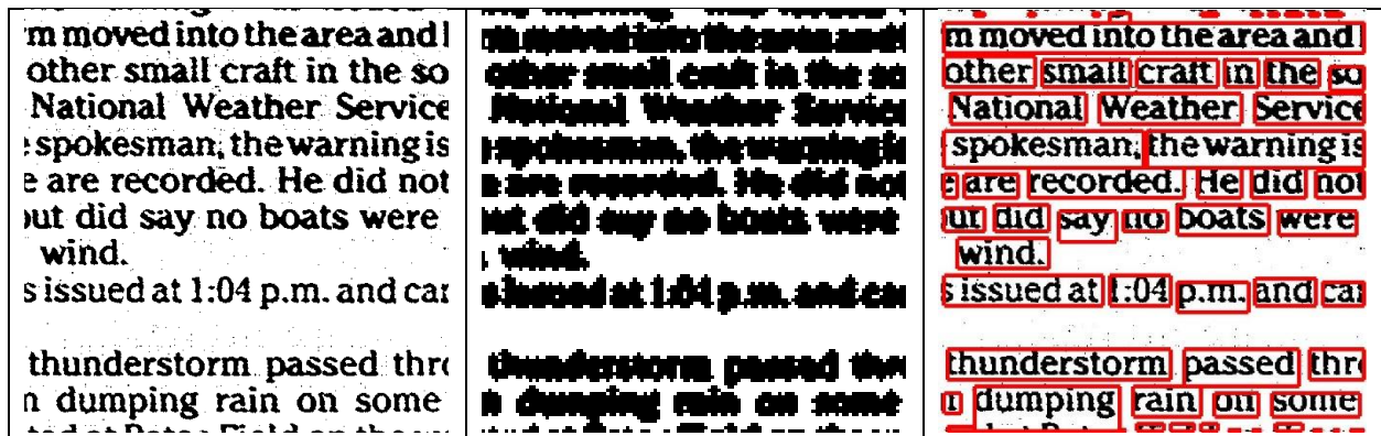
Figure 6: Left image shows original snippet from newspaper. Center image shows results from creating the word blobs. Right images results from creating word zones from word blobs superimposed over original snippet.
