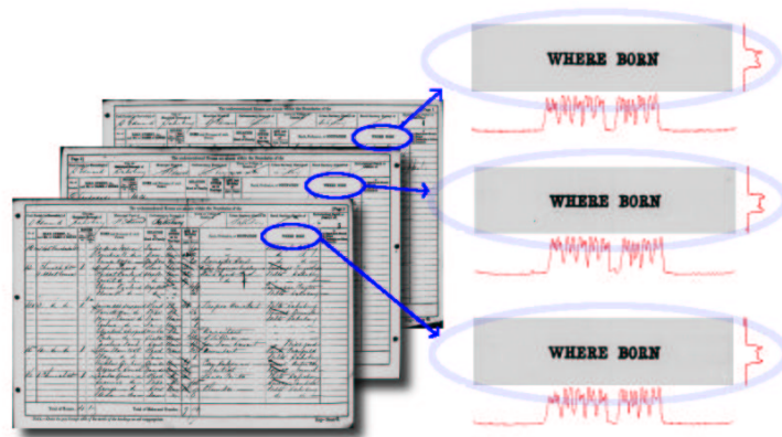
Figure 4: The horizontal and vertical profiles of the same cell in the table from three separate documents
