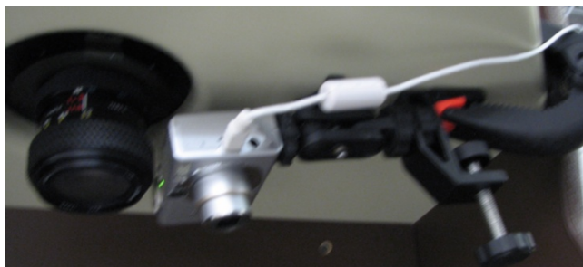
Figure 3: A camera mounted adjacent to the reader lens
