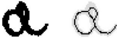
Figure 2. An example of a handwritten lower-case 'a' and its skeleton, obtained by line thinning. Taken from a figure in the paper by L'Homer [8].
