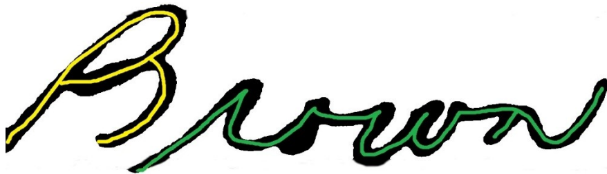
Figure 5i. Once consensus paths are found for D the algorithm continues with whatever was on the stack below S . Consensus paths whose starting points are the endpoints of another path (such as the paths from A, B, C, D, and S) are combined into a single stroke (the yellow path). Consensus paths whose start points are not the end point of another consensus path will be treated as a separate stroke.
