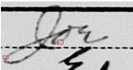
Figure 3a. Handwritten words in scanned documents are often degraded, with low contrast and gaps in the strokes, as highlighted by the red rectangles.
